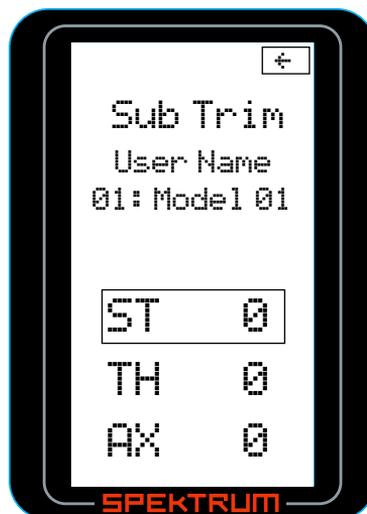
The Sub Trim function is normally used to correct for minor angular inaccuracies that occur when placing the servo horn on the servo. In many cases, the servo horn is not exactly perpendicular to the servo (or in the exact optimum desired position). Minor sub trim values can be used to correct this offset inaccuracy, however, it's important to understand that large sub trim values can limit the total throw of the servo in that direction so small sub trim values only are recommended.
