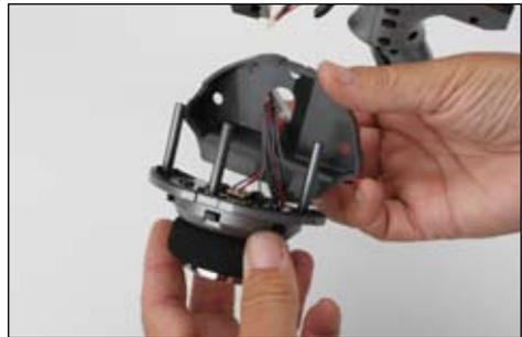
11. Select the opposite “handed” steering shell and pass the steering wheel mechanism connector through the hole in the shell.
