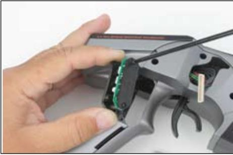
6. Carefully pull out the grip plate that contains buttons D, E and F. Use a Phillips screwdriver remove the PC board and backplate from the grip plate. Note the positions of the three buttons.
