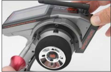
3. Use a 3/32inch hex wrench remove the three screws on the front of the steering housing as shown.
