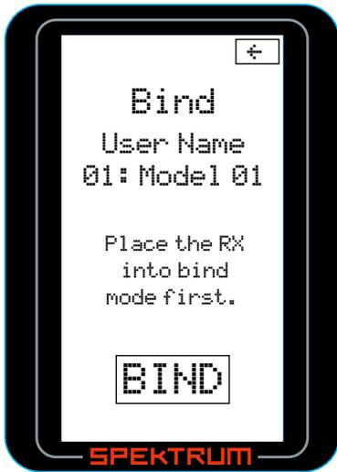
6. Rotate the roller to highlight BIND
