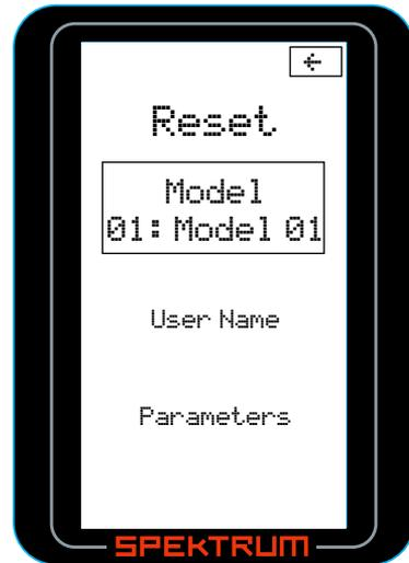
The reset function is used to reset the Model Memory that is selected, the User Name, back to the factory defaults, and the Parameters function is used to recalibrate the transmitter's steering and brake potentiometers.
