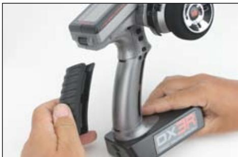
14. Fit the grip in place and reinstall the batteries. Note that the buttons D and E now work in reverse. It will be necessary to change the direction of these switches in the System menu (see page 29)
