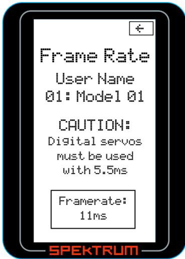
To allow the DX3R to be compatible with all types of servos (older analogs through the latest high response rate digitals), three frame rates are available.
