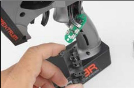
7. Transfer the three buttons (D,E and F) to the other “handed” grip plate noting that the buttons fit in a specific direction such that they fit the external contour of the grip plate.
