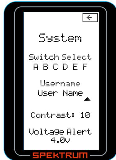
The System function allows the six available switches (A,B,C,D,E and F) to be programmed to the desired function. It allows the user name to be selected, contrast to be adjusted, and the voltage alarm threshold can be set.
