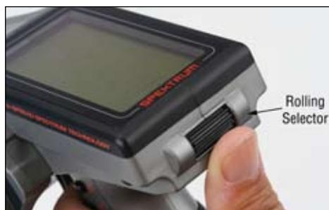
The Rolling Selector is pressed to access functions and rolled to selected specific features or to change setting or values. Pressing and holding the rolling selector for more that 3 seconds returns the display to the main screen.
