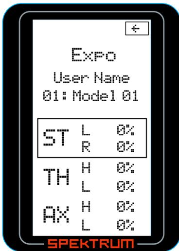
Exponential is used to affect the response rate of the steering, throttle and/ or brake. Typically positive Exponential is used for steering, reducing steering sensitivity around neutral, making it easier to drive the car at high speeds in a straight line but exponential still allows for the maximum turning radius.
