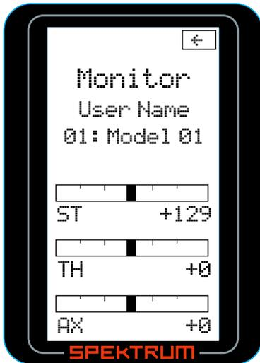
A servo monitor is available that displays the servo output positions graphically and digitally. This monitor can be useful in troubleshooting setups, displaying mixing functions and how they interrelate, etc.
