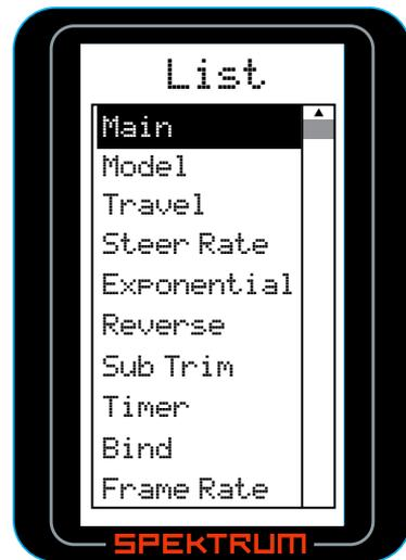
The List screen displays all the available functions. The desired function can be accessed by highlighting the desired function using the roller and when highlighted, press the roller to enter the function.
