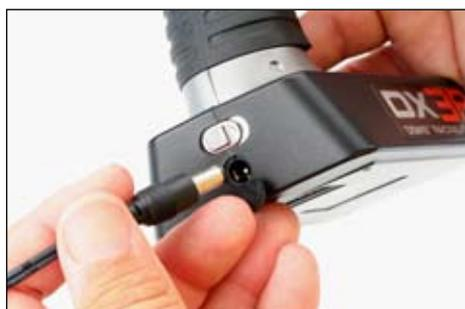
A charging jack is located just below the on/ off switch. If rechargeable batteries are used, they can be conveniently charged without removing them from the transmitter using the charge jack.
