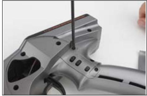
9. Place both grip plates in place and fasten them using four Phillips screws (two per side).
