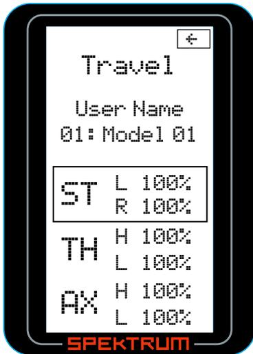
The Travel screen (sometimes referred to as travel adjust or end points) allows independent travel adjustment of the servo throw in each direction of all three channels (steering, throttle and auxiliary). A graphic illustration displays the effect of travel adjust.
