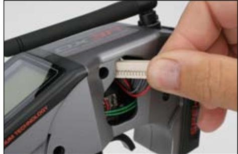
10. Push the steering wheel connector through the transmitter case to the opposite side.
