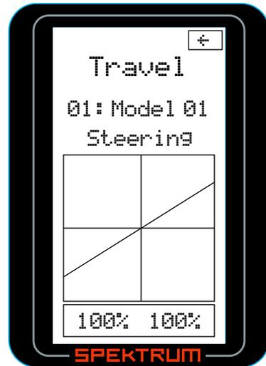
Rotate the roller to highlight the values at the bottom of the screen; then press the roller to select the values.
