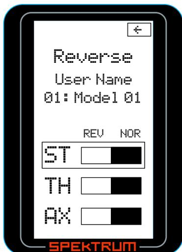
The Reverse function (also known as servo reverse) establishes the servo's direction relative to the channels input (i.e. a right steering input should result in a right steering angle at the car). Reverse is available on all three channels and is normally the first function that is checked and adjusted during programming.
