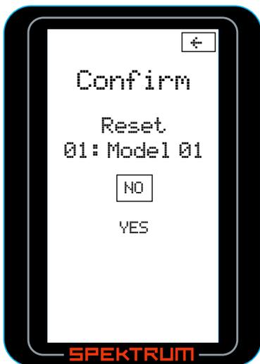
Use the roller to highlight YES; then press the roller to reset.
