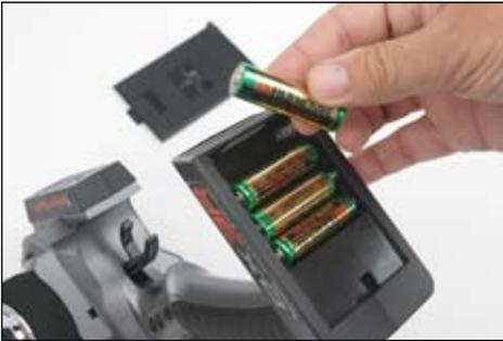
1. Remove the batteries from the transmitter. This prevents the possibility of accidentally causing a short during the conversion.
