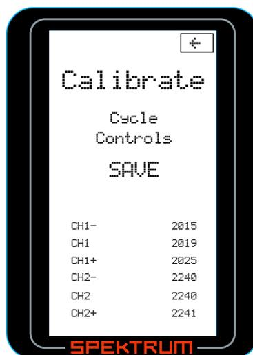
Rotate the steering wheel full right then full left; then move the throttle trigger to full throttle and full brake. Note: The values will change to correlate with the actual potentiometers.
