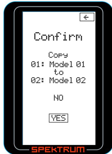
If the selected model is correct, use the roller to highlight YES and press the roller to copy from the current model to the selected model.
