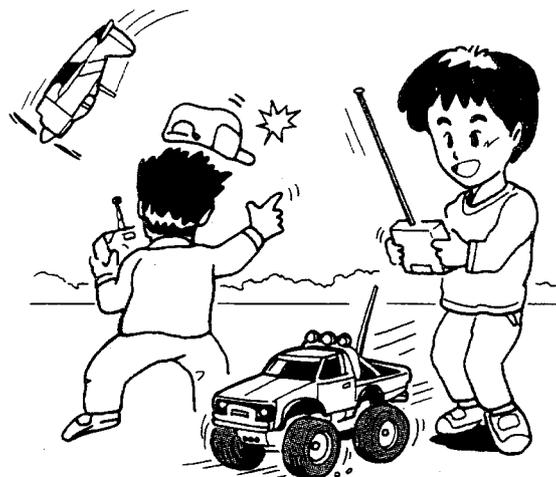
Make sure that no one else is using the same frequency as yours in your running area. Using the same frequency at the same time, whether it is driving, flying or sailing, can cause loss of control of the R/C models, resulting in serious accidents.
